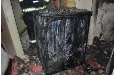
Lack of maintenance is the leading cause of dryer fires. Clothes dryers must vent hot air to the outside of the house. If lint builds up in the exhaust vent or inside and around the dryer, it can block the flow of air causing the dryer to perform poorly, raising the operating temperature of the dryer and causing it to overheat.
